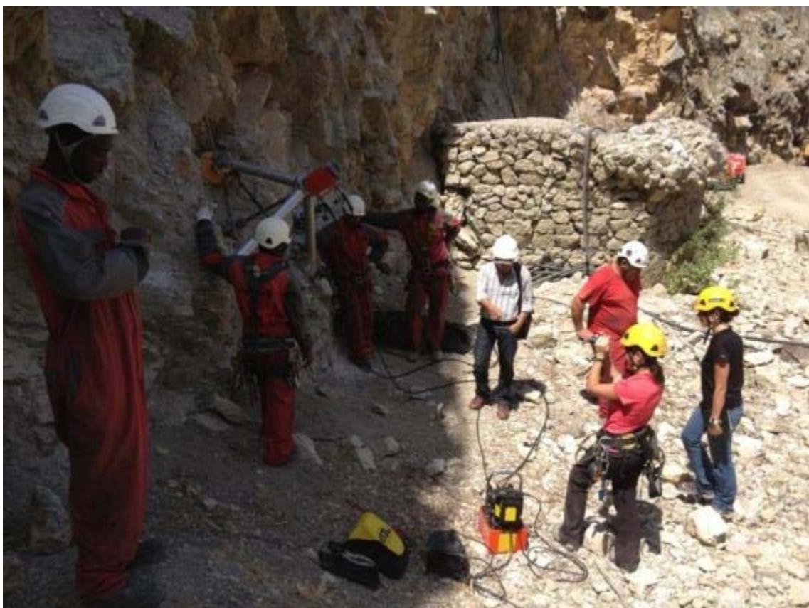
Picture 42:Tensile tests
